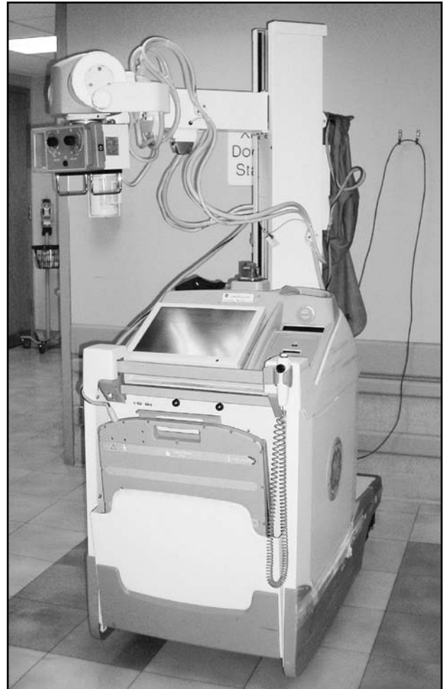
Figure 5. Portable x-ray machine with 6-ft exposure cord and hook for lead apron.
