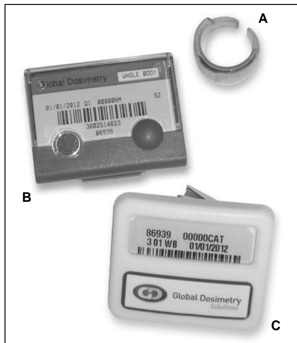
Figure 1. Ring badge (A), thermoluminescent dosimeter (B), and film badge (C).
